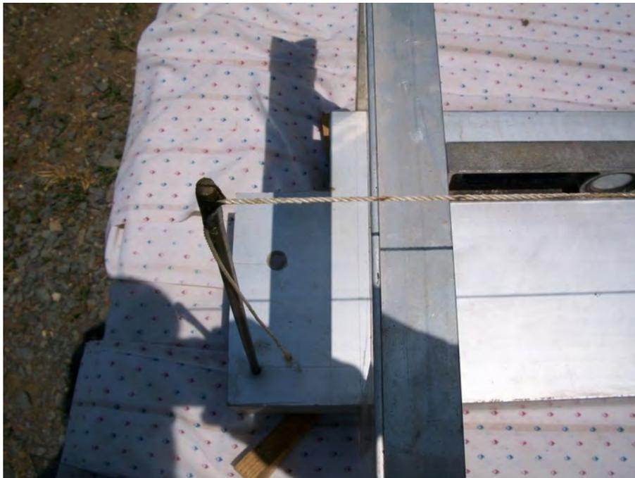
In the picture to the left, notice that the 'third' piece of aluminum which was in first picture and on table is now placed directly on top of the 'plumb' two uprights which are north/south. Edges matching! I used 90 degree material for the uprights and 'cross-bar' for strength and aligning purpose.
