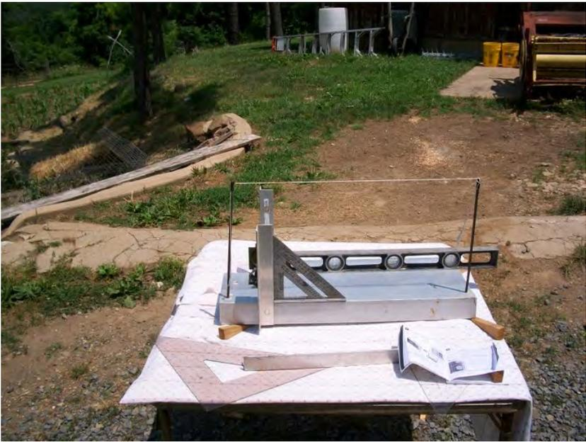
The materials must be non-magnetic. Aluminum used in this case with 2 inch sides for attaching uprights. Notice 'square' to 'plumb' uprights. Notice 'level' to level aluminum platform - both ways. North and West. Notice 'wooden wedges' to level platform.
